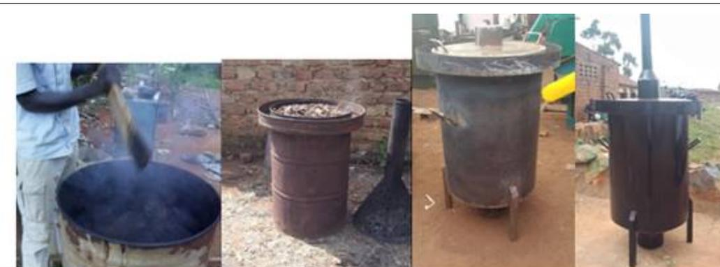
**Figure 3. Metallic drums showing the modifications**
